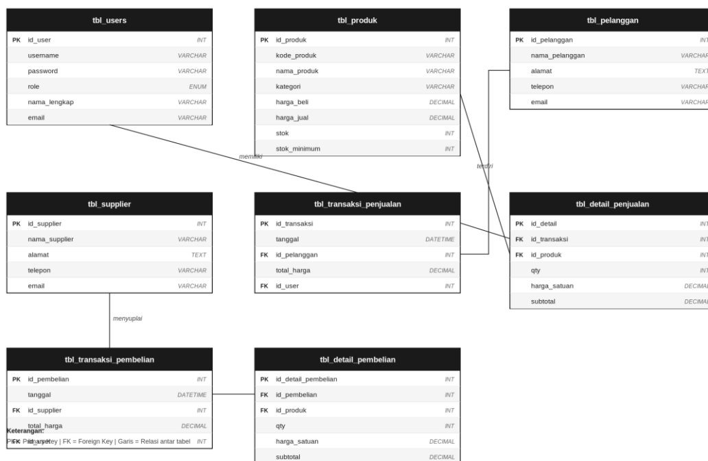
Gbr. 3. Entity Relationship Diagram delapan tabel database sistem.
